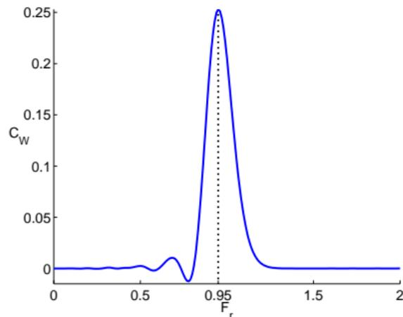
Wave resistance coefficient  $C_W$  at time  $T = 10$ , depending on the Froude number  $Fr$ , with  $\delta = 1$  and  $2$  ( $\gamma = 0.9$ ,  $\varepsilon = 0.1$ ).
